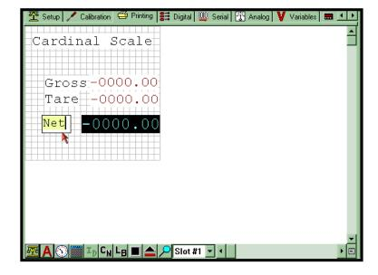
Notice on this label we have added time and date to this label/ticket. The time has been applied and now we are adding the date. We have clicked on the calendar button from the selections from the bottom of the screen and are positioning it in the area right below the time. Notice that the Net Weight print has been inverted to put emphasis on the final weight for the customer.
