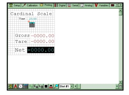
Drawing lines and creating boxes is easy. Just select the small black box button from the bottom of the screen and place it in the label area. (restricted to thermal printers only) You can drag the wand, as shown, to adjust line thickness and length..
