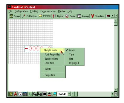
To create static text, click and drag the "A" button from the bottom of the screen to the label/ticket. Double click on the box that will appear and type the desired text. After typing the text, right click on the text box to change the font, inverted print, and print rotation. Note that weight does not have a description until you create the text box beside it. You have complete control with nControl<sup>TM</sup>!
