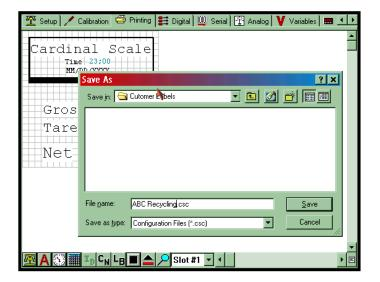
You can send the label/ticket directly to the printer or to the indicator. Select printing and click on the proper selection as shown in this picture. The transfer to the indicator utilizes a standard RS-232 cable and should be connected to serial port 1 of the 205/210 indicator. This is a bi-directional port. Export will send this current ticket to an external file. Import allows you to search and choose from all exported ticket files.
